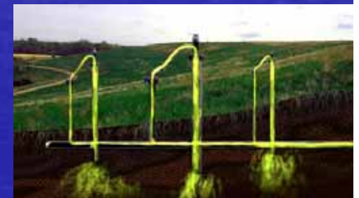
LFG Wells and Collection Piping
