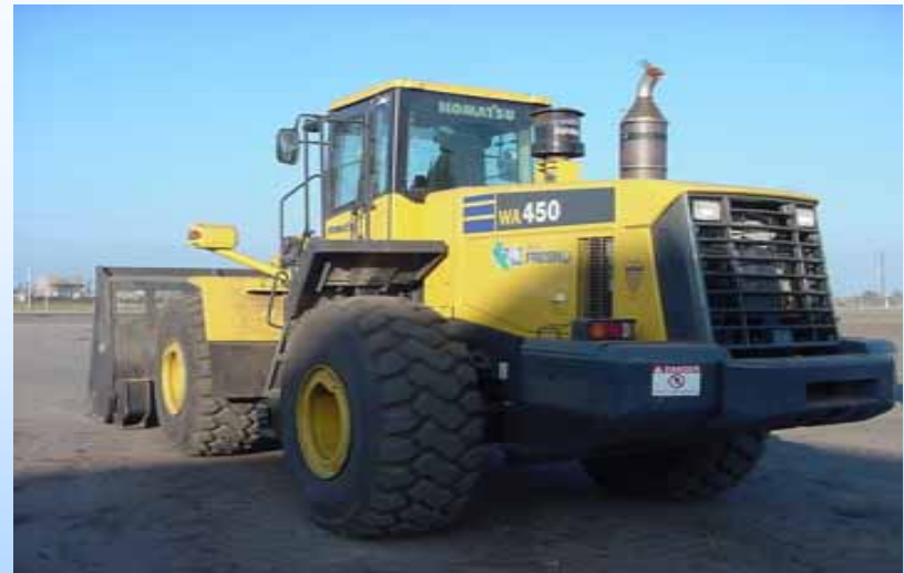
DPF Retrofit (ref: West Coast Collaborative)
